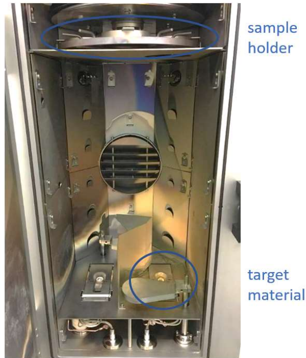
Figure 11: Vacuum chamber of a Winter Vakuumtechnik HVB 130 showing the target material and the sample holder positioned above.
