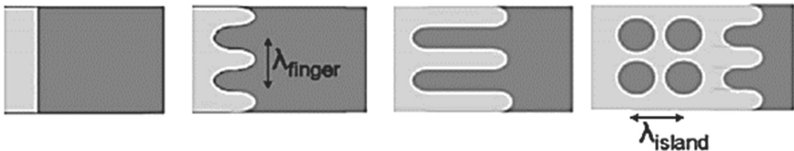
Figure 4: Top view of the fingering process evolving into islands due to Rayleigh instabilities [1].
